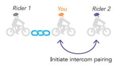
In a 4-way intercom conference call, for example, you are connected to three riders, who may also be connected to an additional rider. You are directly connected to Rider 1 and Rider 2, and connected to Rider 3 through Rider 2's free channel. All four riders are now all connected in a 4-way Bluetooth intercom call.
